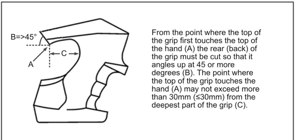
From the point where the top of the grip first touches the top of the hand (A) the rear (back) of the grip must be cut so that it angles up at 45 or more degrees (B). The point where the top of the grip touches the hand (A) may not exceed more than 30mm ( $\leq 30\text{mm}$ ) from the deepest part of the grip (C).
